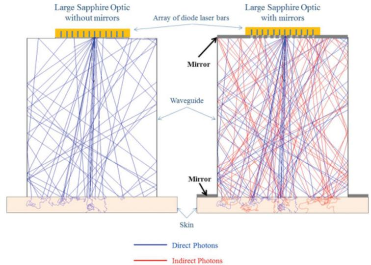
**FIGURE 3** Cross-sectional view of Large Sapphire Optic waveguide on skin with results of a Monte Carlo ray trace model shows the benefit of the photon recycling mirrors. For the same incident fluence, there is a gain of 1.5 X in the number of photons at a target in the skin with the addition of the mirrors.
